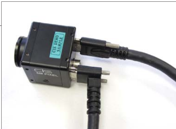
Kinking of a cable must be avoided at all times and properly designed strain reliefs will help to prevent this from occurring. Source: Nortech Systems
