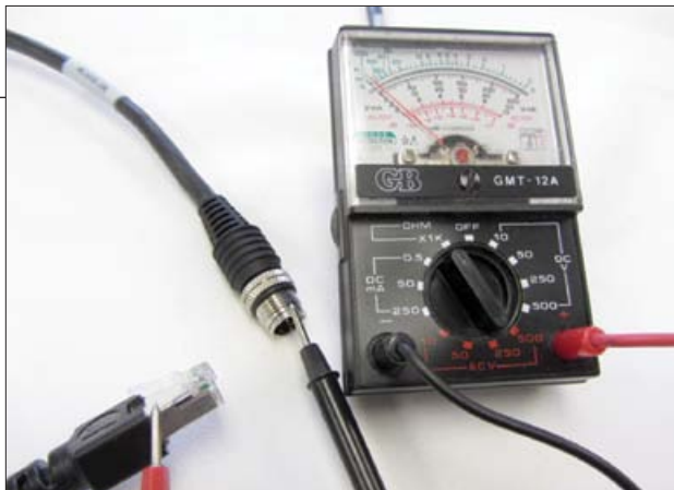
A simple continuity test can be performed by touching one probe to the threaded metal body of the M12 connector and the other probe to the metal shield on the RJ45 connector. The presence of electrical continuity indicates a properly designed and terminated assembly. Source: Nortech Systems
